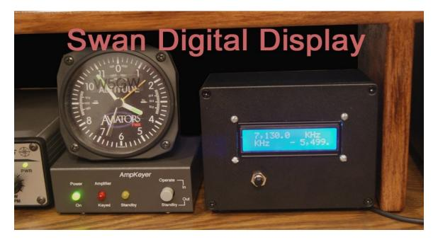
This display unit could have been built much smaller, but I happened to have this nice enclosure available. With this display I can easily monitor my frequency. While my Swan's accuracy and stability is not on a par with my modern gear, the addition of a digital display makes operation and changing frequency (QSYing) much easier.
